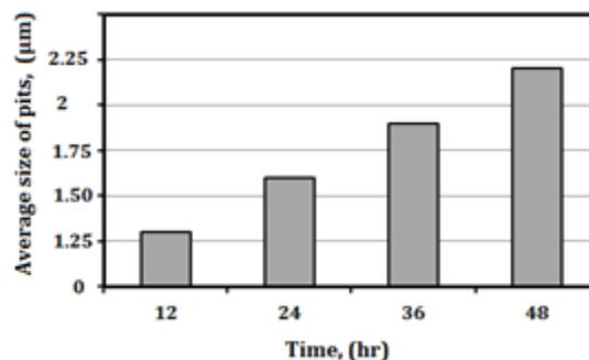
**Figure 8: Histogram of the Average Size of Surface Pits vs Testing Time that Formed After E-C Tests for AA 6066 Alloy**
