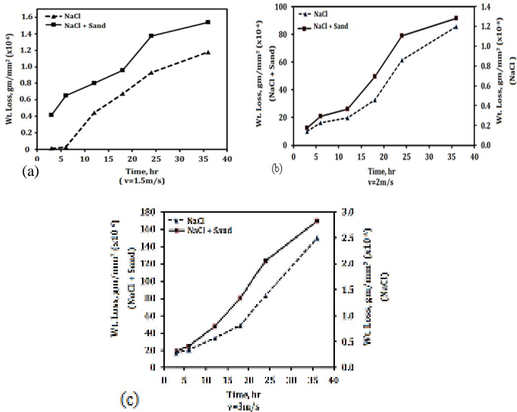
Figure 2: Weight-Loss vs Testing Time for AA 6066 Alloy Tested in NaCl Solution and NaCl Solution with 20 wt.% Sand Particles; a) Velocity: 1.5 m/s, b) Velocity: 2 m/s and c) Velocity: 3 m/s
