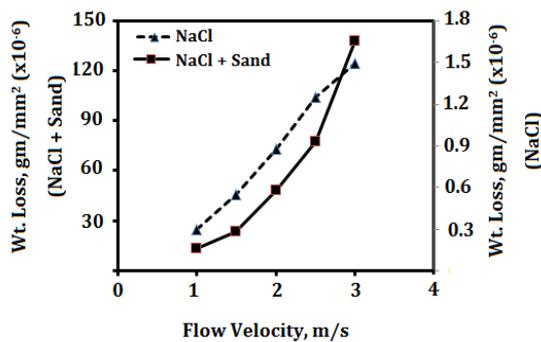
Figure 3: Weight-Loss vs Flow Velocity of Specimens of AA 6066 Alloy. All Specimens Were Tested for 24 Hrs and a Velocity 2 m/s
