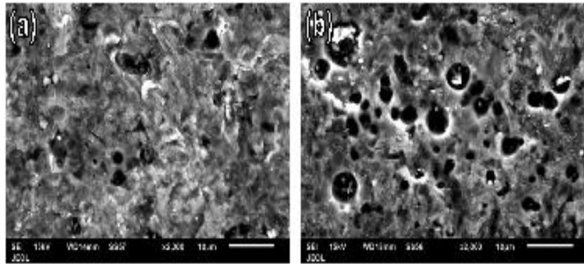
**Figure 7: Typical SEM Micrographs of Eroded-Corroded Surface of Specimens of AA 6066 Alloy, at High Magnification (x2000); (a) Tested for 36 Hrs and (b) Tested for 48 Hrs**
