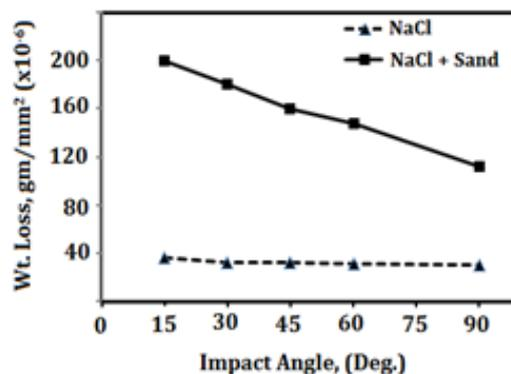
Figure 5: Weight-Loss per Unit Area vs Impact Angle for Specimens of AA 6066 Alloy Tested for 24 Hrs in NaCl Solution with 20 wt. % Sand Particles, and Flow Velocity of 2 m/s
