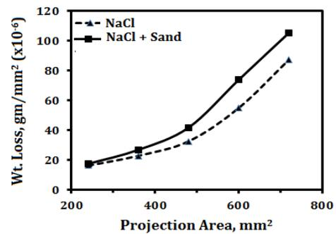
Figure 4: Weight-Loss vs the Projected Areas of Specimens of AA 6066 Alloy. All Specimens Were Tested for 24 Hrs and a Velocity 2 m/s
