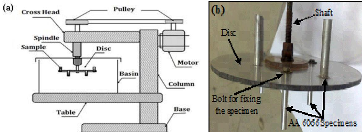
**Figure 1: a) A Schematic Draw of the Test Rig Used in the Present Study and b) Optical Photo of the Polymeric Disc Used for Fixing the Test Specimens**
