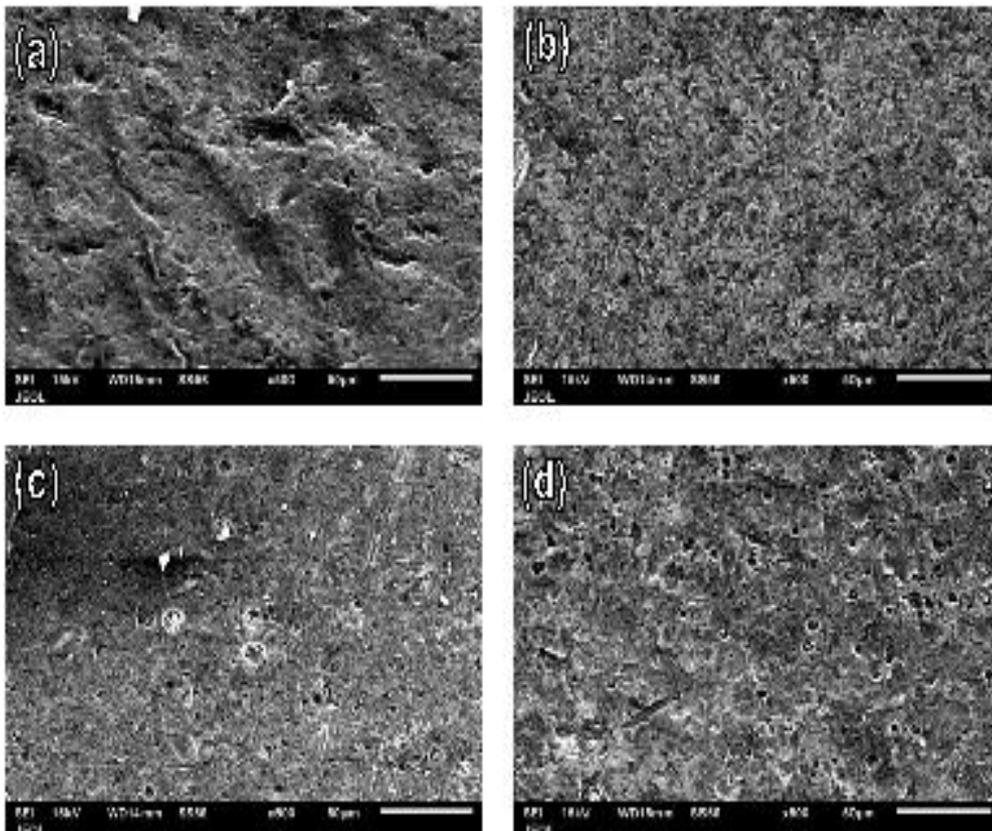
**Figure 6: SEM Micrographs of Eroded-Corroded Surfaces of Specimens of AA 6066 Alloy Under Different Testing Times (x500); (a) for 12 Hrs, (b) for 24 Hrs, (c) for 36 Hrs, and (d) for 48 Hrs**
